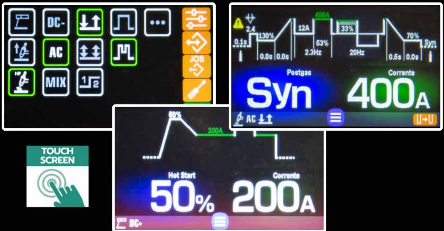
**ENG** • Thanks to the **touchscreen technology**, welding parameters can be set quickly and easily. It is however possible to set the machine using the two knobs on the panel. 3 user interface modes: Basic, Intermediate and Advanced.
